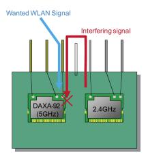
One DAXA-92 and one 2.4GHz wifi module can work simultaneously (dual band dual con-current, DBDC) in the same platform under different frequency band, DAXA-92 in 5GHz and the other WiFi module in 2.4GHz, without Rx sensitivity degradation.
