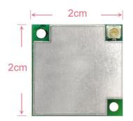
RM5 is an IEEE802.11b/g wifi proprietary CF module in 2.0cm x 2.0cm small form factor designed specifically for integration in application-specific devices (ASDs) used in vertical market. RM5 has Bluetooth coexistence function by directly connect to Bluetooth with another two control signals and no extra pull high /low resistor required. It provides the highest flexibility and extensibility to implement WiFi/ Bluetooth coexistence.
